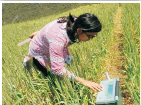
Fig.44. Field measurements of gas exchange parameters using a portable photosynthesis system (LICOR).
