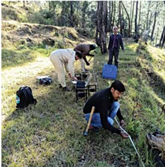
Fig. 3: Geophysical resistivity survey in Devalikhan recharge zone
