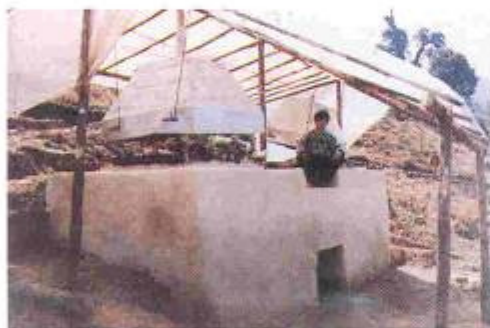
Fig. 1. Twin-kiln prototype for large cardamom curing designed at Pangthang
