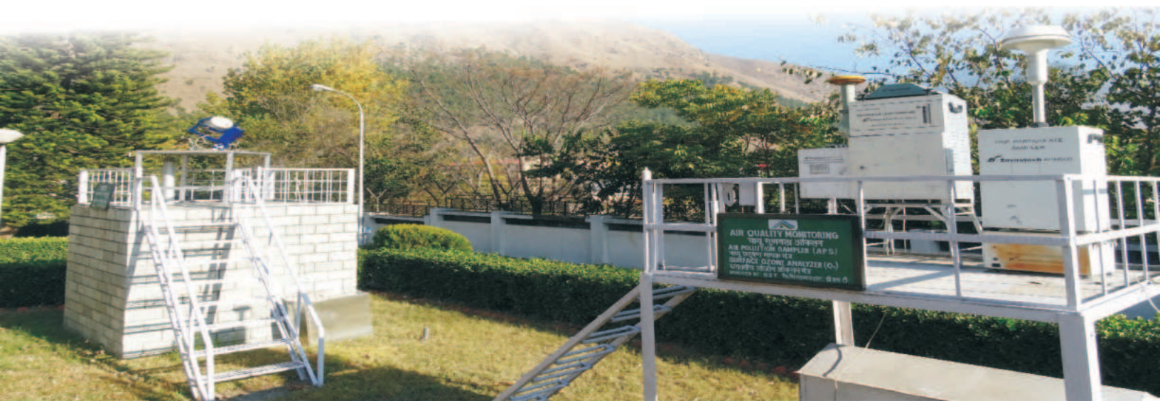
Fig. 34: Multi-wavelength Radiometer (MWR) and Respirable Dust Sampler (RDS) set ups for aerosol and particulate matter measurements at Mohal, Kullu (H.P.).
