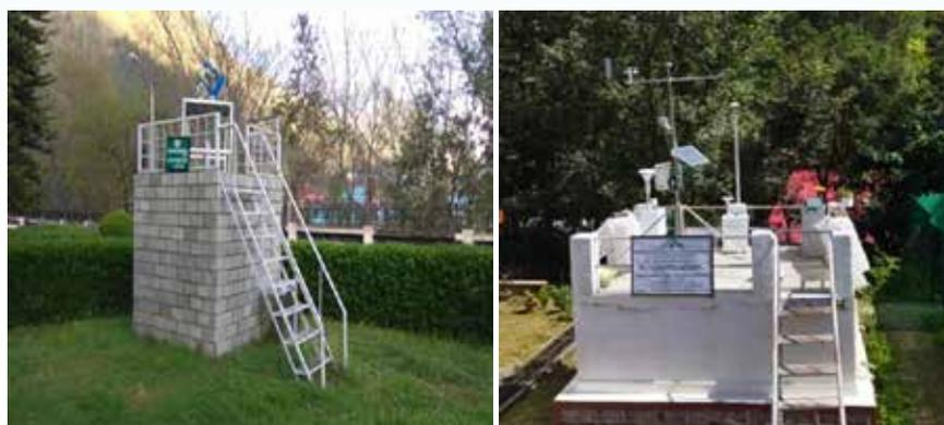
**Fig. 31:** (a) Multi-wavelength radiometer (MWR) set up for aerosol measurements at Mohal (b) Air quality monitoring station at Kosi-Katarmal, Almora
